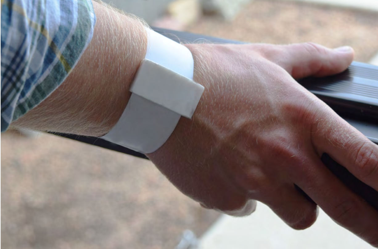
The Wanderguard door controller is connected to a sensor based bracelet on a resident's arm.
